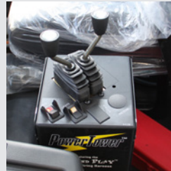
Inside air controls mounted in ergonomic power tower featuring Plug And Play™ wiring
