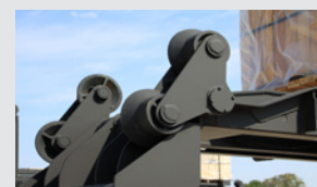
Dual rear rollers are ductile cast iron 6" OD and flared sides w/ bronze bushing
