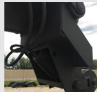
Rear hydraulic activated stabilizer with 10" ground roller
