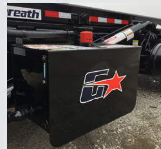
50-gallon steel hydraulic tank side mounted with dual sight / temp gauge
