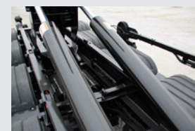
In frame rail rollers and bronze bushings allow for smooth loading / unloading
