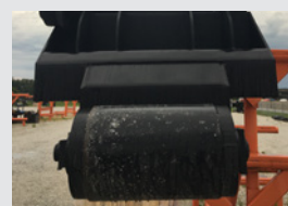
Rear hydraulic activated stabilizer with 10" ground roller
