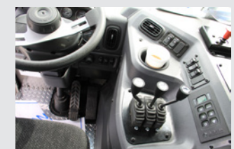
Inside air controls center mounted in ergonomic Power Tower featuring Plug And Play™ wiring. (Top) traditional cab, (bottom) cab over
