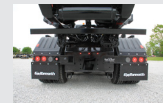
HD rear apron pintle ready with split bumper and LED lighting
