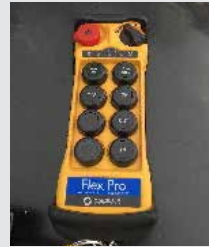
Electric over hydraulic operation using a wireless remote control (8-button w/ emergency stop)
