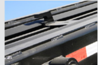
Single stationary rear hold down inside of frame rails
