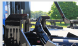
Raised Front Stops w/ Knuckle Cable End and Dual Automatic Spring Loaded Pass Over Front Container Safety Locks
