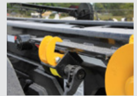
Auxiliary Front Container Stops; Rear Wing Skid Plates and Nylon Ratchet Hold Downs
