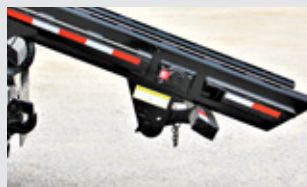
Auto folding air assist ICC bumper (standard on OR, IO, OX models); auto folding mechanical ICC bumper (standard on IX models)
