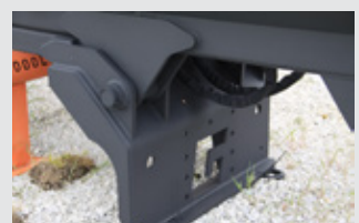
HD lowered rear hinge with pintle adaptable rear apron
