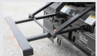
Auto folding air assist ICC bumper (standard on OR, IO, OX models); auto folding mechanical ICC bumper (standard on IX models)
