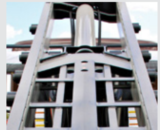
Single cylinder winch rail w/ rod protector
