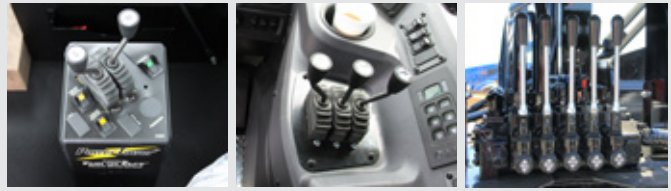
Inside air controls in power tower or integrated into center console on cab over trucks; secondary outside manual controls at main control valve
