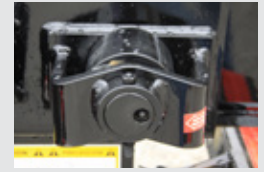
4" O.D. Outboard supported side rollers
