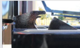
Automatic spring loaded pass over front container safety lock
