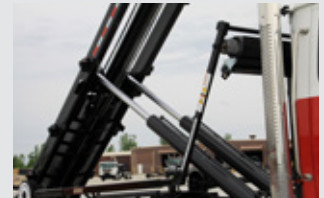
Reverse mount, inboard above frame lift cylinders
