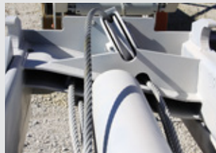
Offset front sheave assembly w/ 10" grease grooved cable sheaves
