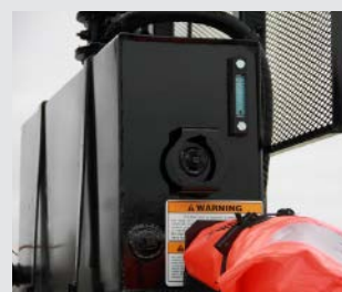
BTC oil reservoir with dual site/temperature gauge.
