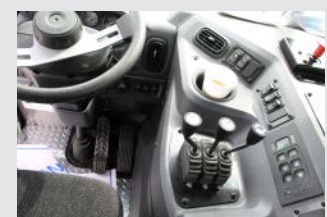
Inside air controls center mounted in ergonomic Power Tower featuring Plug And Play™ wiring. (Top) traditional cab, (bottom) cab over.
