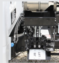
Secondary outside manual control valve with protective cover
