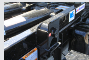
Welded & bolted on roller stools with 4" OD rollers & bronze bushings
