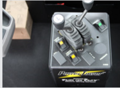
Inside air controls in power tower
