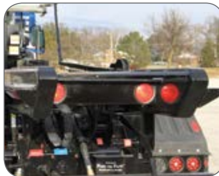
Rear cross members with California compliant lighting.
