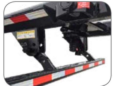
Air assist ICC bumper standard on most cable hoists models (not required on HH, EX, EH, IX models).
