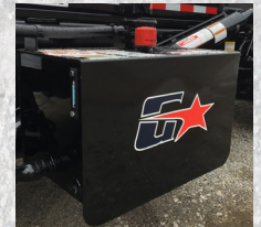
50-Gallon steel hyd. tank w/ dual sight/temp. gauge (U30/U3-DPHK)
