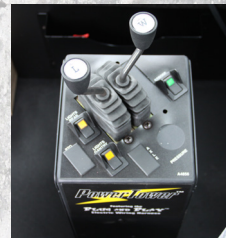
Inside air controls in power tower
